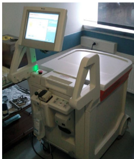
Fig. 1 Automatic infusion system used in Department of Nuclear Medicine at University Medical Centre in Ljubljana
